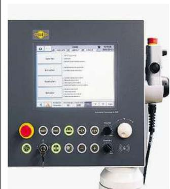
functions for flat grinding. These range from flute, face and creep-feed grinding to grinding-disc and program management or profile dressing.
