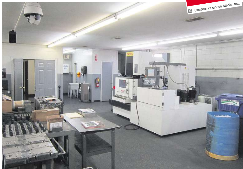
LED cameras are positioned to view a machine's control screen or workzone enable users to see if a tool or EDM wire has broken.
