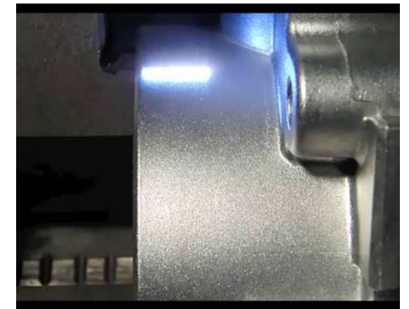
Removal of dirt and structuring of the surface
