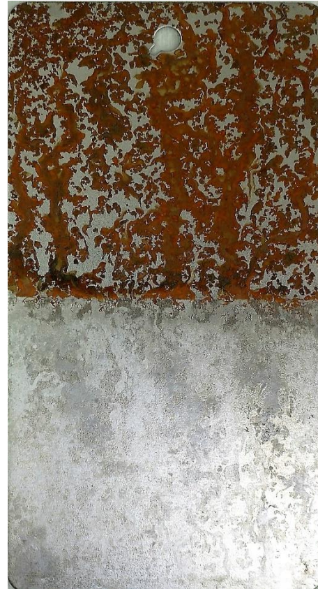
Rust removal 3 min, 10%, 45°C
