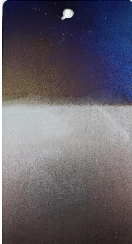
Scale removal 1 min, 10%, 45°C
