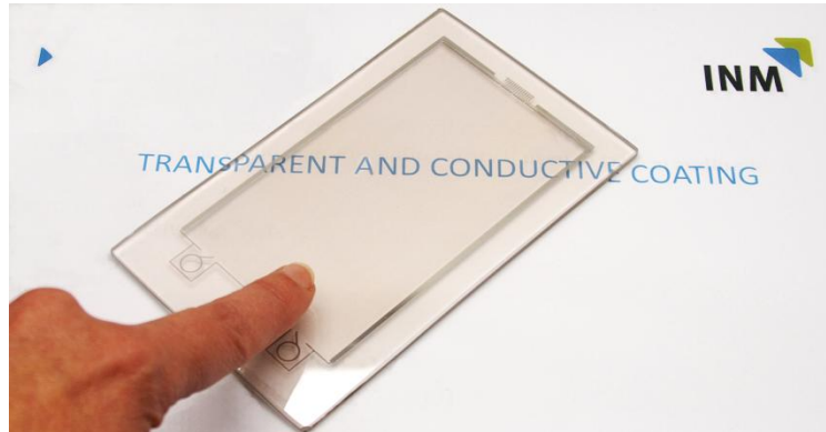
silver mesh touch panel structure on glass
