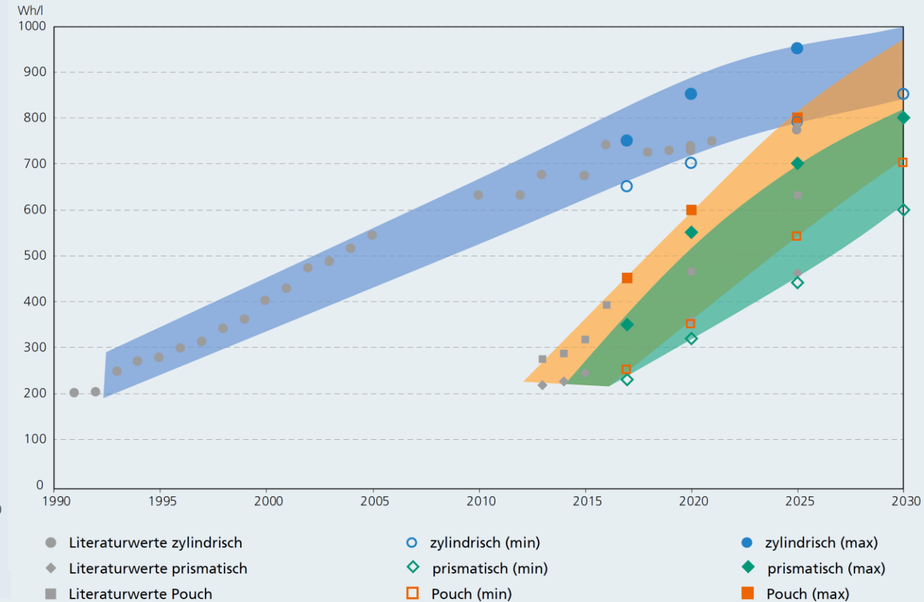
Development of vol. energy density (Wh/l) for LIB cells by cell format (cylindrical, prismatic, pouch)
