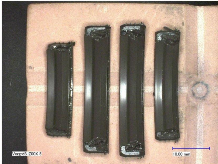
Test 1: Engine oil (10W-40) without REWITEC®
