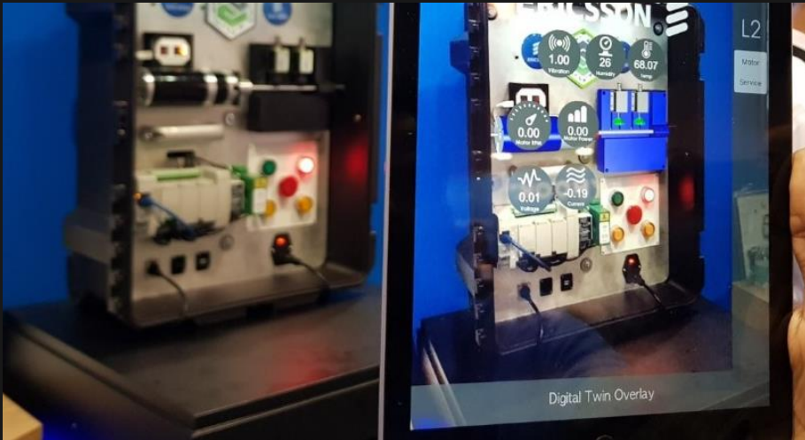
Digital twin inspection
