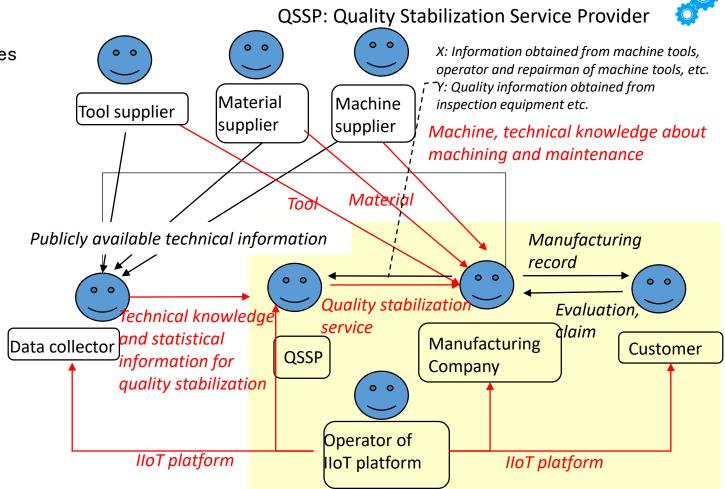
Data collector, who collects public information from a number of parties and provides summary and analysis results via service platform, plays a central role. IIoT platform used by a quality stabilization service provider can be different from that used by data collectors and other parties.
