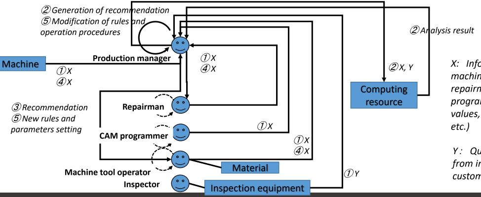
X: Information obtained from machine tools, operator and repairman of machine tools, and CAM programmer (conditions, parameter values, details of executed actions, etc.)
