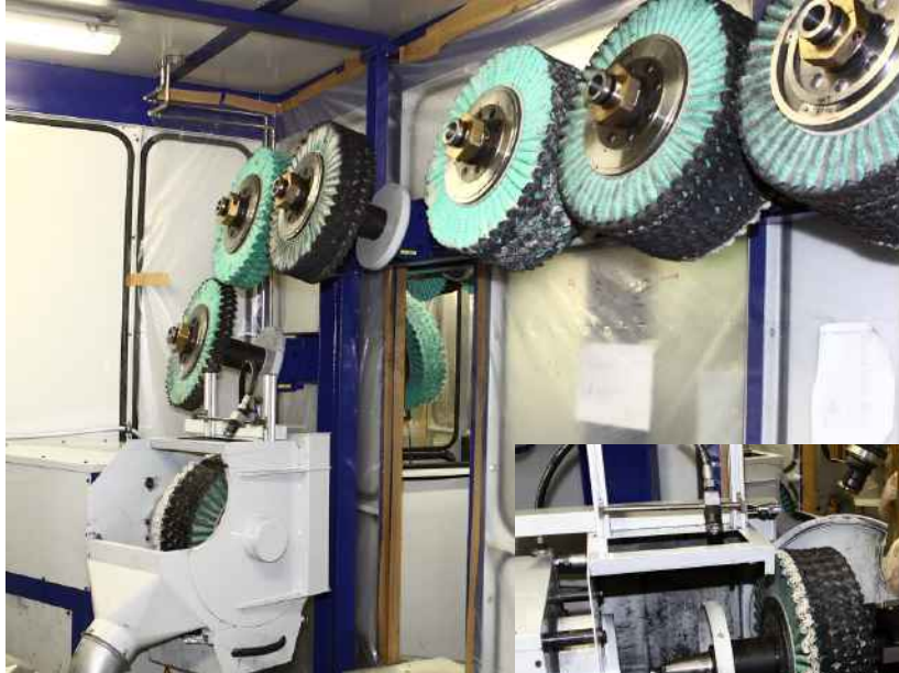
Robot polishing system with automatic tool and gripper exchange system
