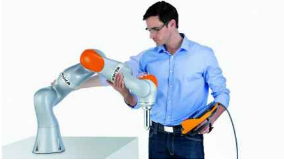
Kuka robot type IIWA with measuring system for forces and moments in every robot axis Reference: Kuka Robotics
