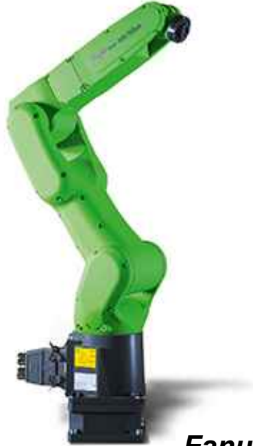
Fanuc robot with measuring system for forces and moments in the base of the robot Reference: Fanuc Robotics
