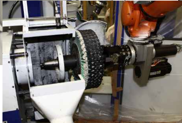
Robot polishing system with automatic tool and gripper exchange system
