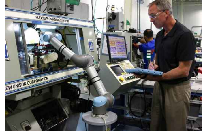
Universal Robot with measuring system for forces and moments Reference: UR Robotics
