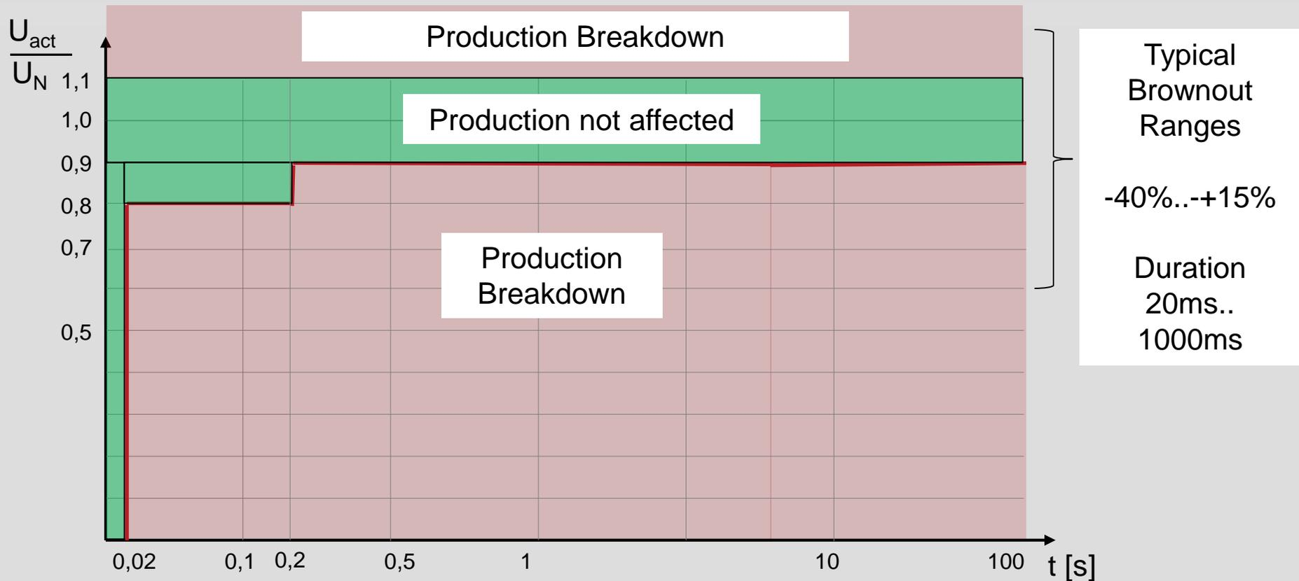
Local Voltage drop, voltage disturbance by harmonics may minize the operational safety !!!
