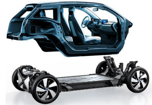
BMW i3 - Composite-metal hybrid concept (Source: BMW AG)
