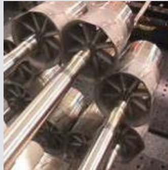
DLN/ULN Burner: <15-25ppm NOx
