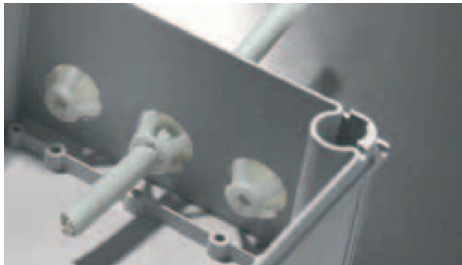
The membrane cable entry Wiska Clixx combines the advantages of a membrane grommet with those of a cable gland.
