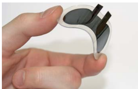
Printed battery comprising two cells in series (3 Volt)
