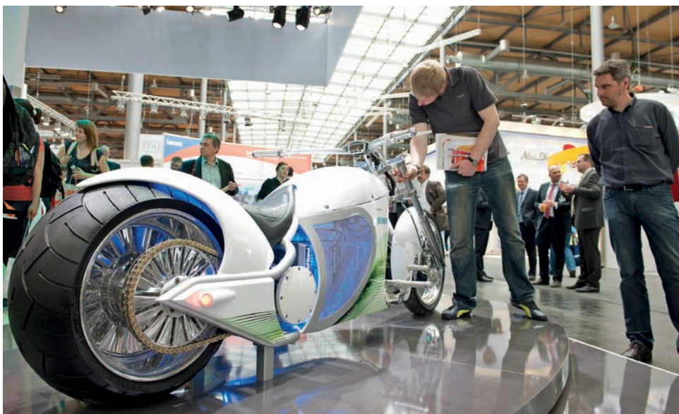
This Siemens bike is powered by an electric motor. It has a range of around 80 kilometers (50 miles) per charge.
