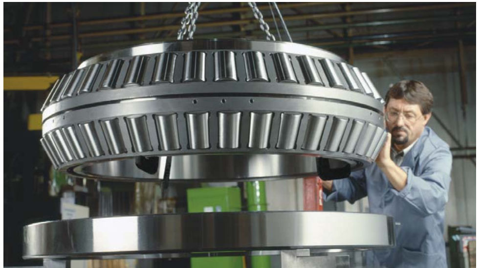
Assembly of a tapered roller bearing for a wind turbine rotor.
