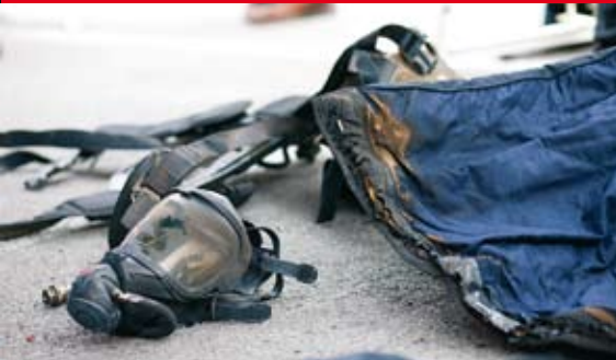
Left: “Thermo Man” undergoing a fire test Below: The charred remnants of a protective suit
