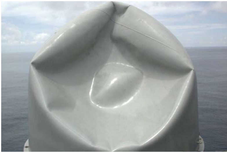
TV-DTS Antenna's Close Encounter with AC Exhaust Plume
