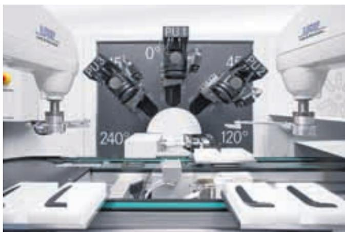
The new LPKF Fusion 3D laser structurer directs up to four lasers onto the component from seven possible positions.
